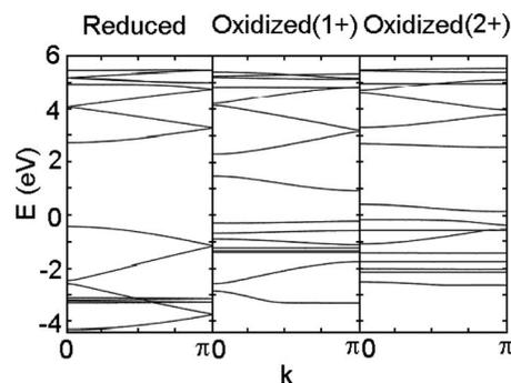
FIG. 7. Electronic band structure of infinite chains of reduced and oxidized PPy.
