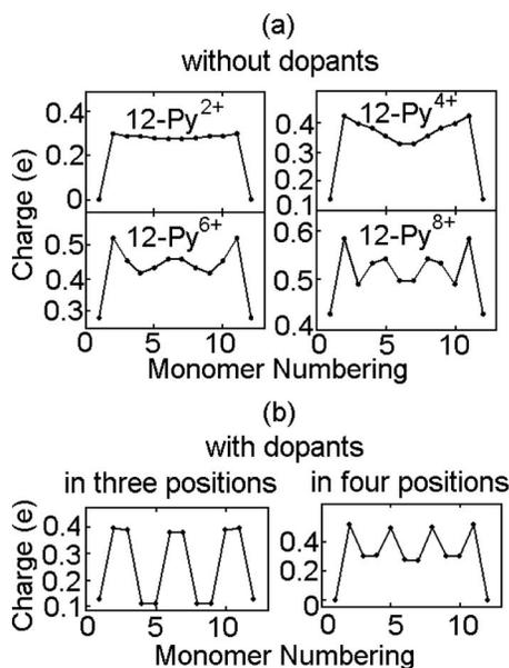
FIG. 6. Distribution of charge per monomer along the backbone of oxidized 12-Py. (a) Various oxidation levels and (b) charge localization due to dopants.
