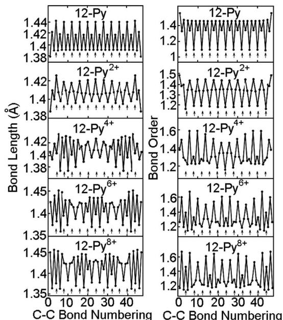
FIG. 4. Distribution of bond lengths and bond orders along the backbone of reduced and oxidized 12-Py. Arrows mark the position of the C—C inter-ring bonds.
