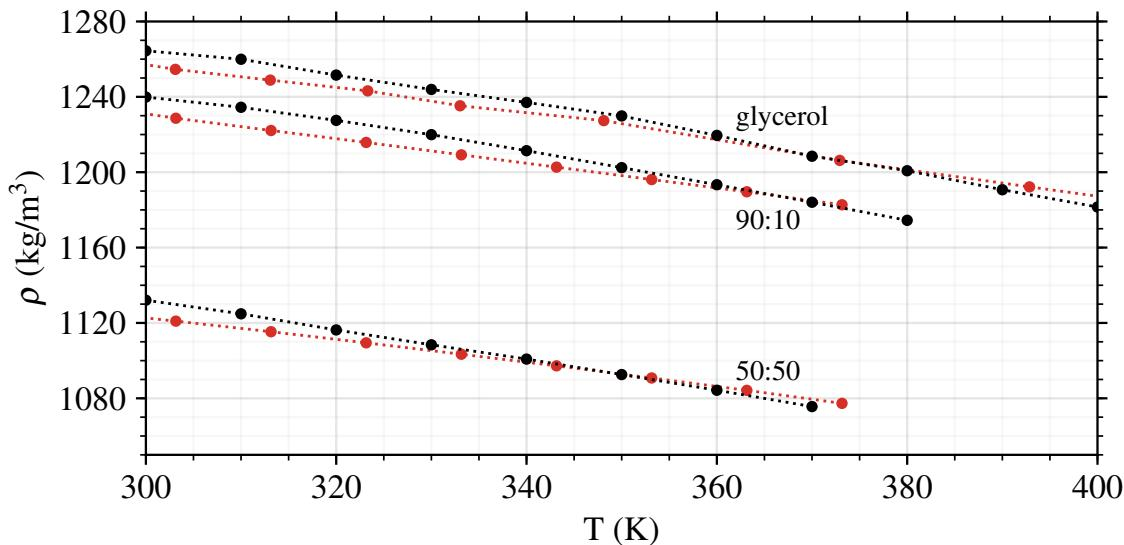
**Figure S1.** MD simulated densities of pure glycerol and two glycerol:water mixtures of 90:10 and 50:50 (depicted black) are compared to experimental measurements (depicted red) from *Gregory, S. R. (1963). Physical Properties of Glycerine and its Solutions (Glycerine Producers' Association).*
